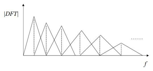
Figure 5.5: Example of triangular filters used to compute MFCCs. (Image From: Jinjin Ye: Speech Recognition Using Time Domain Features from Phase Space Reconstructions, MSc thesis, (2004))
