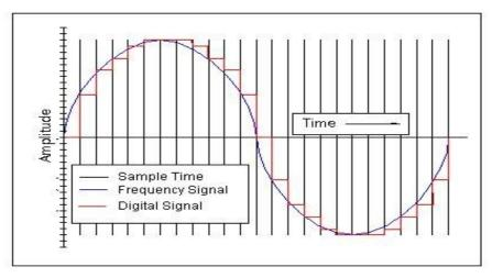
**Figure 2.6:** From analog signal to digital. First we convert the analog signal to a discrete-time signal via sampling, and then, to digital via quantization (Image from: http://www.soneti.net/csp/digital%20signal.JPG)
